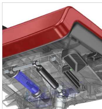
Gas lift controls the speed of the tilt return
